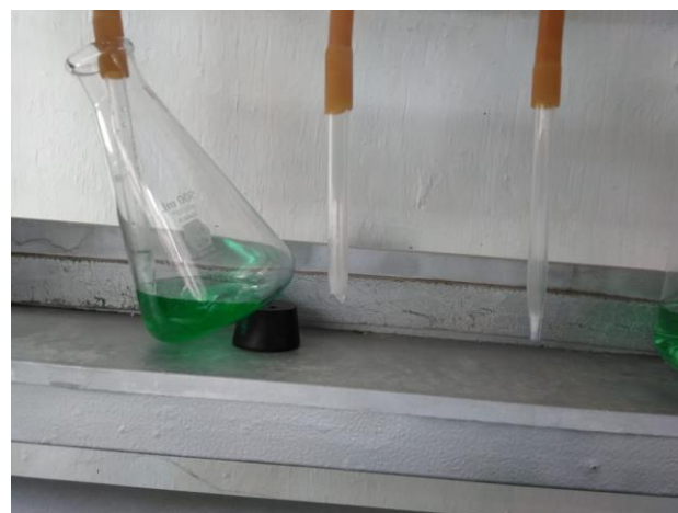
Figure 2 Determination of crude protein by the Kjeldahl method
