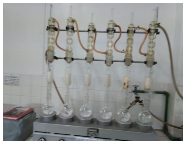
Figure 3 Soxhlet apparatus for determination of raw fat
